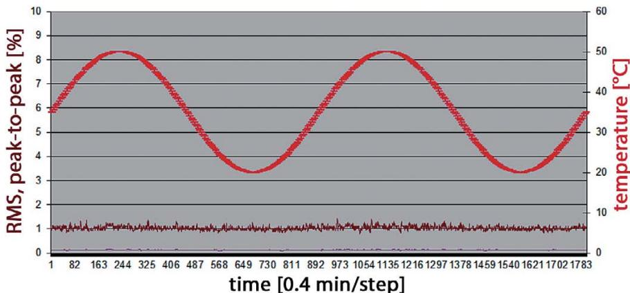
**Figure 5: Typical long-term intensity noise of a 594 nm DPSS-laser as a function of temperature at thermal cycles from 20 to 50°C in 12 hour periods**
