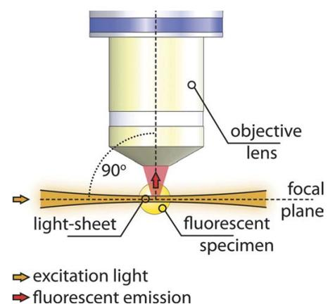
**Figure 1: Functional principle of a light sheet fluorescence microscope. Fluorophores in the embryo are illuminated from the side with a just a few  $\mu\text{m}$  thick light sheet. The emitted photons are collected by the detection lens perpendicular to the illumination plane. The focal plane of this lens coincides with the illumination plane**
