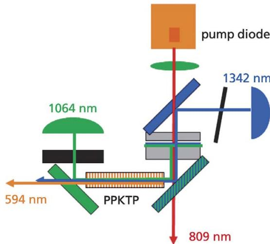
**Figure 4: Functional principle of a DPSS laser with sum-frequency generation of 594 nm in a PPKTP crystal**
