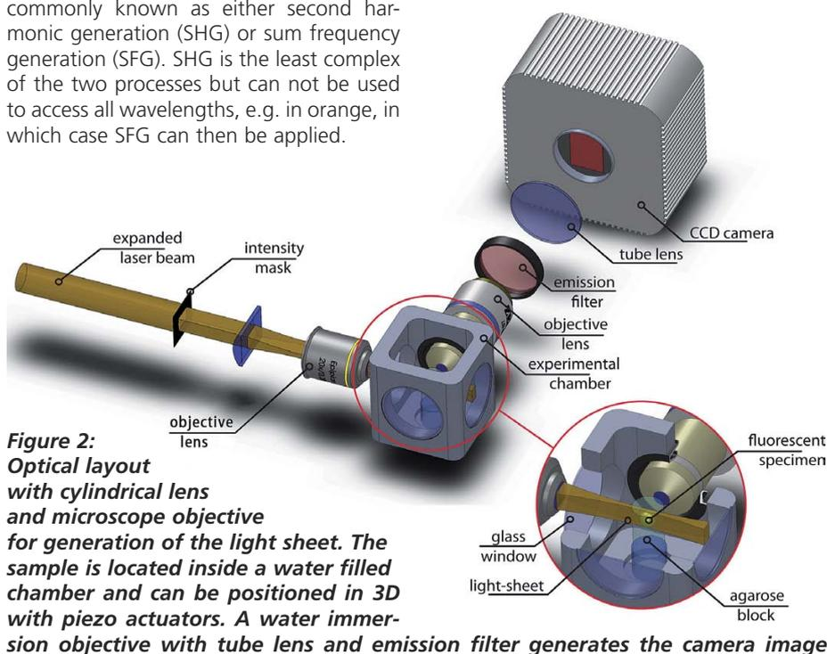
**Figure 2:** Optical layout with cylindrical lens and microscope objective for generation of the light sheet. The sample is located inside a water filled chamber and can be positioned in 3D with piezo actuators. A water immersion objective with tube lens and emission filter generates the camera image
