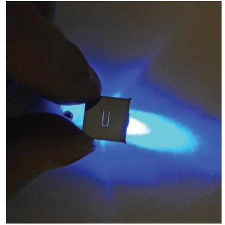
Figure 1. Silicon MEMS-fabricated cantilever pressure sensor.
