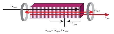
Figure 3. Schematics of signal-resonant OPO based on a quasi-phase-matching (QPM) nonlinear optical crystal.
