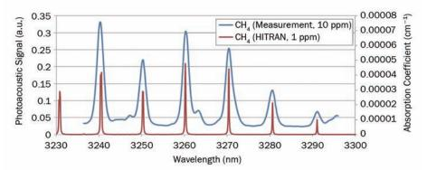
Figure 7. 10 ppm of CH<sub>4</sub> measured with OPO/CE-PAS, with 3.3-ppb detection limit at 1-s integration time.
