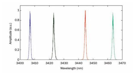
Figure 4. Continuous spectral tuning of the Cobolt Odin OPO over 60 nm.
