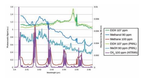
Figure 9. OPO/CE-PAS measurement of EtOH, MeOH and CH<sub>4</sub>.
