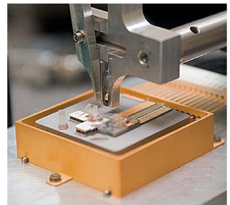
**Figure 1: Laser pre-assembly (left) and active alignment of optical components with  $\mu\text{m}$  precision (right), prior to permanent fixation using high temperature curing technology**
